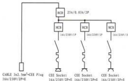
Figure 2 A06MA01-4 assembly configure of electrical principle
